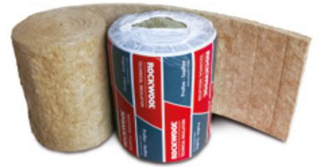
ProRox BL 938<sup>SA</sup> is a blanket type product used in thermal insulation of non-vibrating industrial equipment's where temperatures can be up to 350 deg Celcius. It is easy to install for large diameter vessel.
